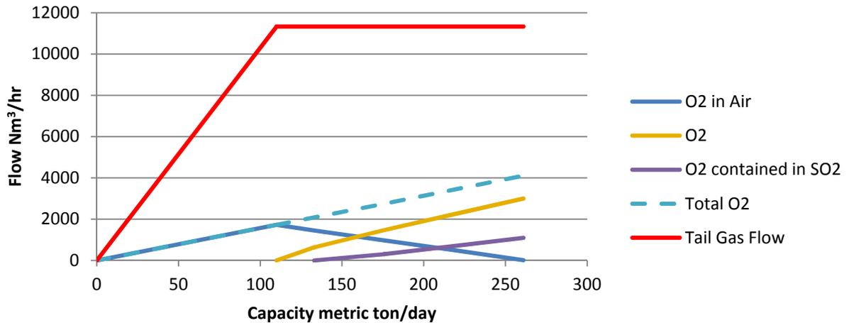
The amount of oxygen required to convert H<sub>2</sub>S to sulfur and water vapor is the same regardless of whether the oxygen comes from combustion air, supplemental oxygen, or oxygen already combined as sulfur dioxide. (Ignoring possible minor effects of dissociation of H<sub>2</sub>S at higher temperature).
