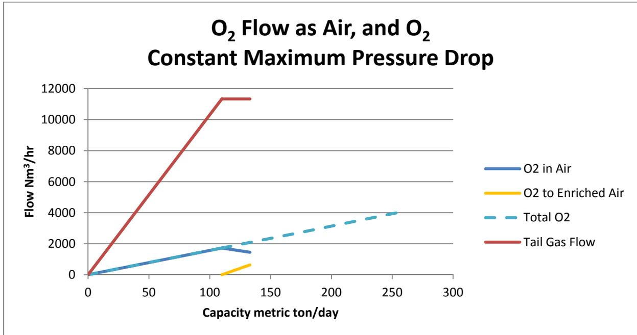
As oxygen is added to the system and air is removed, the temperature inside the reaction furnace increases. A limited amount of oxygen can be added before reaction furnace refractory limitations are reached. To add more oxygen (and remove more air) the temperature rise must be controlled. This is done by adding a mix of sulfur dioxide and oxygen rather than just oxygen.
